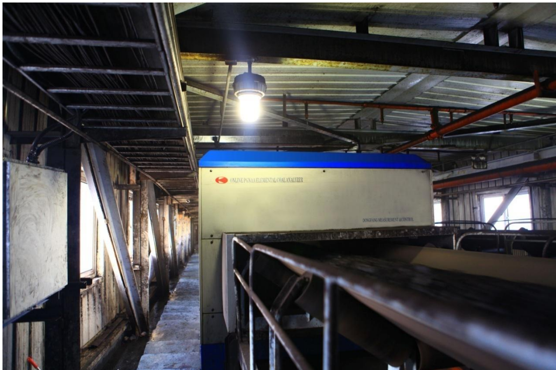
Huadian Jinshan Thermal Power Company Analyzer Application of Coal into the Furnace
